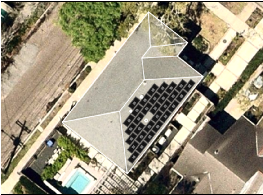
Composite of roof plan-view and array layout
