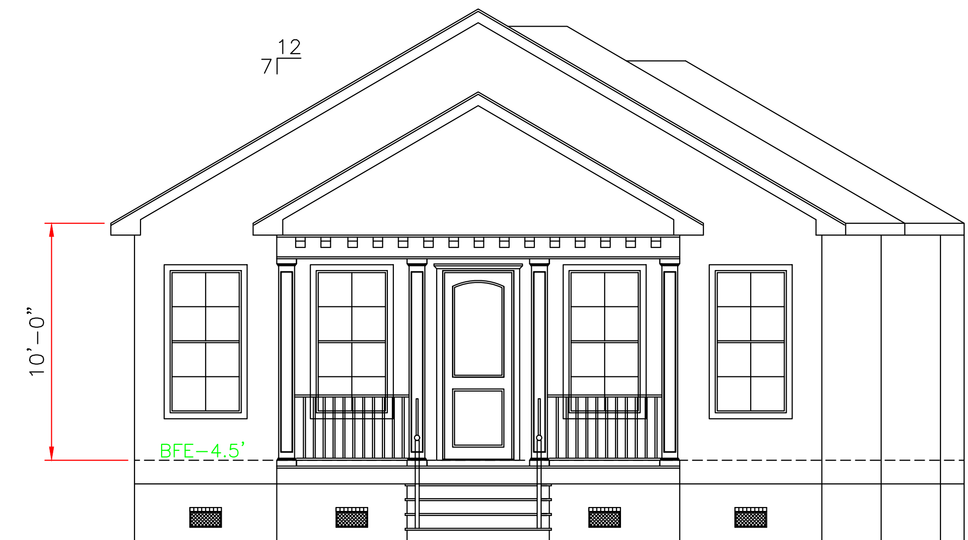
OPTION A FRONT ELEVATION SCALE: 1/4" = 1'-0"
