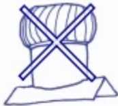
Turbine Ventilator Not appropriate – Can only be installed as a replacement in-kind
