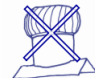
Turbine Ventilator Not appropriate – Can only be installed as a replacement in-kind
