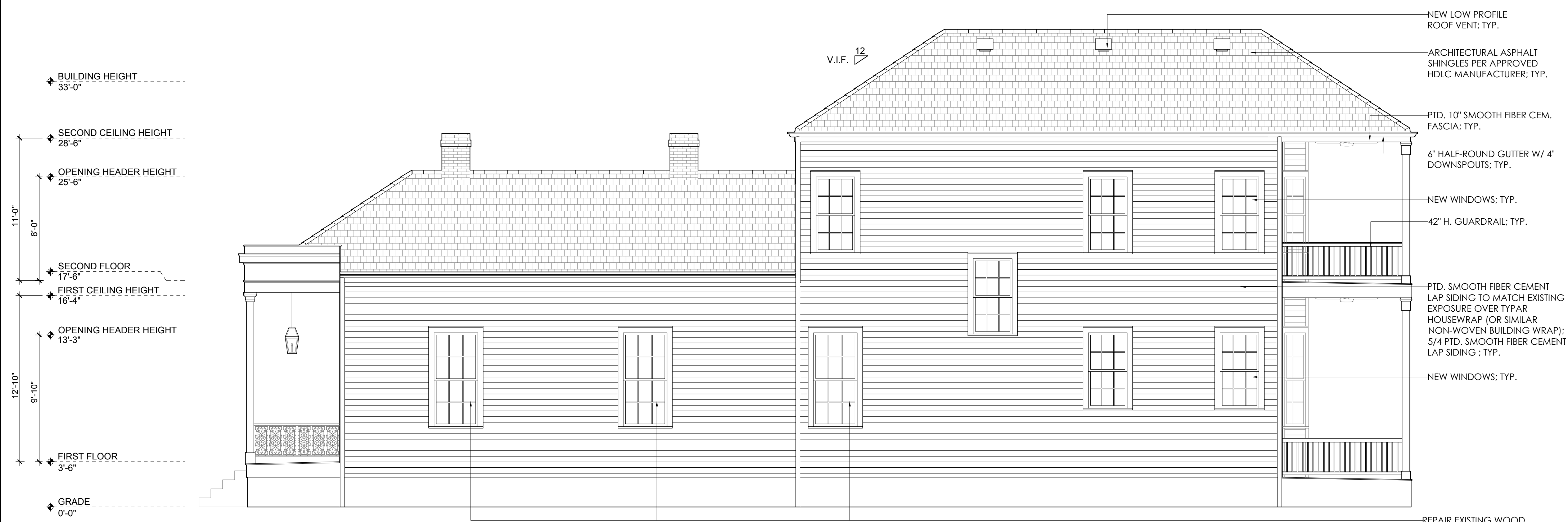
03 WASHINGTON AVENUE (SIDE) ELEVATION SCALE: 3/16" = 1'-0"
