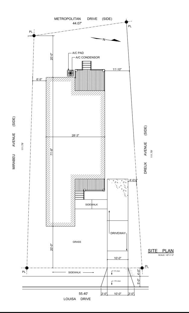
Design Code: IRC 2015 Wind Load: 130 MPH
