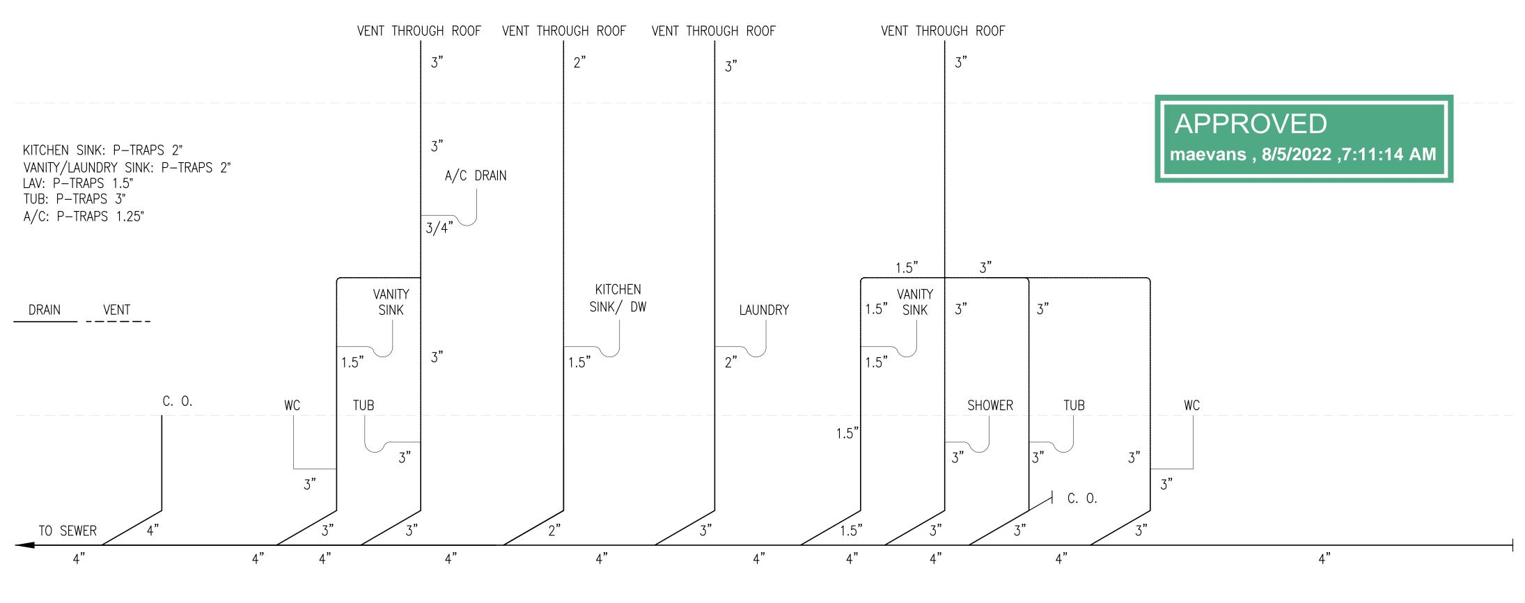
PLUMBING RISER DIAGRAM SCALE – 3/8" = 1'0"
