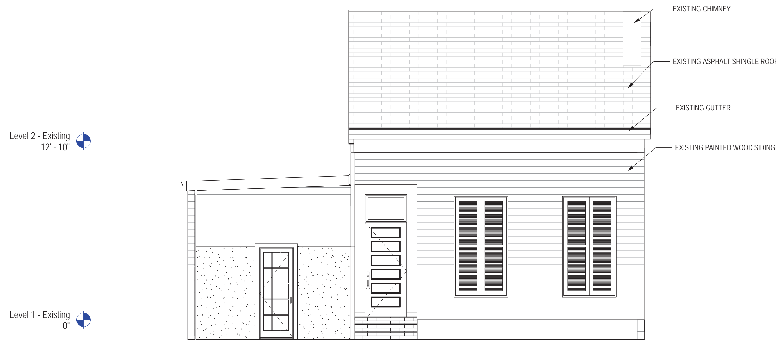
1 A201 Existing Elevation - St Anthony St Side 1/4" = 1'-0"
