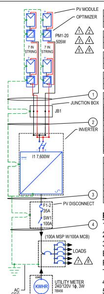
AC Solar disconnecting means will be adjacent to the utility meter
