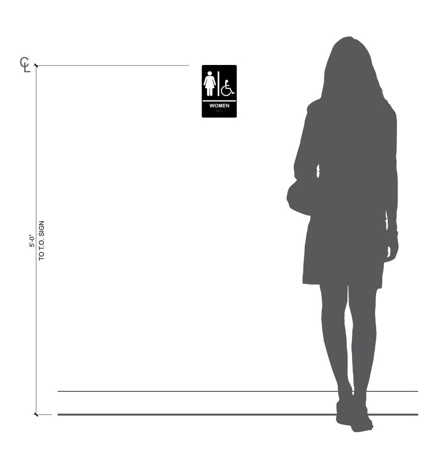
**O2**RESTROOM SIGNAGE -TYPICAL ELEVATION SCALE: 1 1/2" = 1' - 0"
