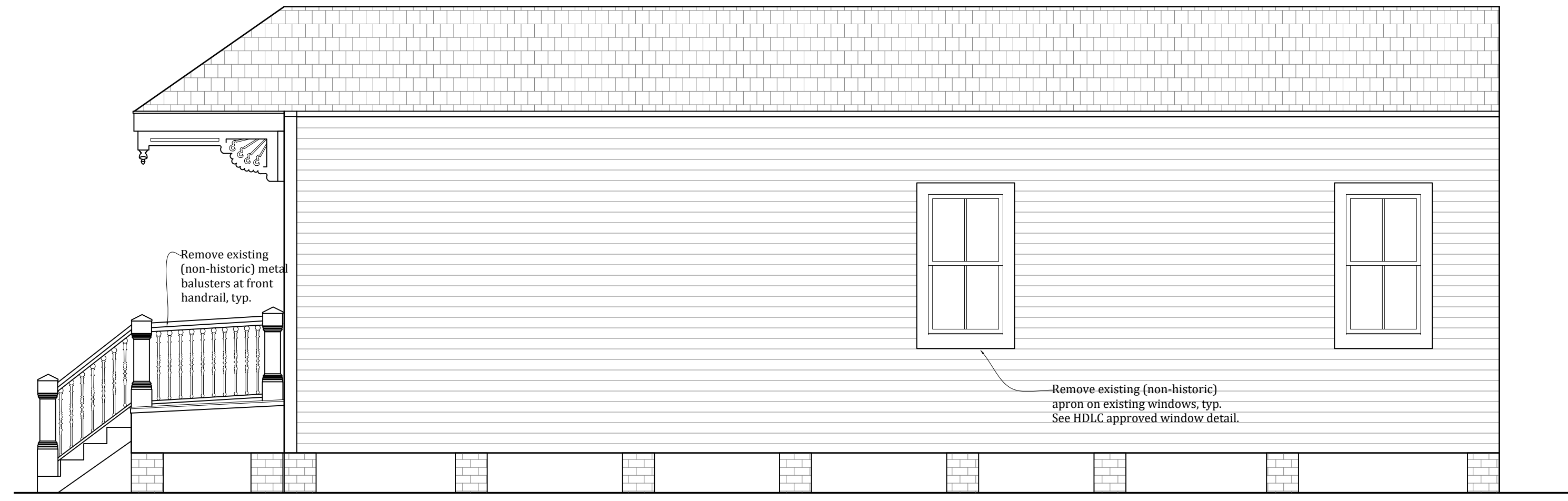
Existing Right Side Elevation Scale: 3/16" = 1'-0"
