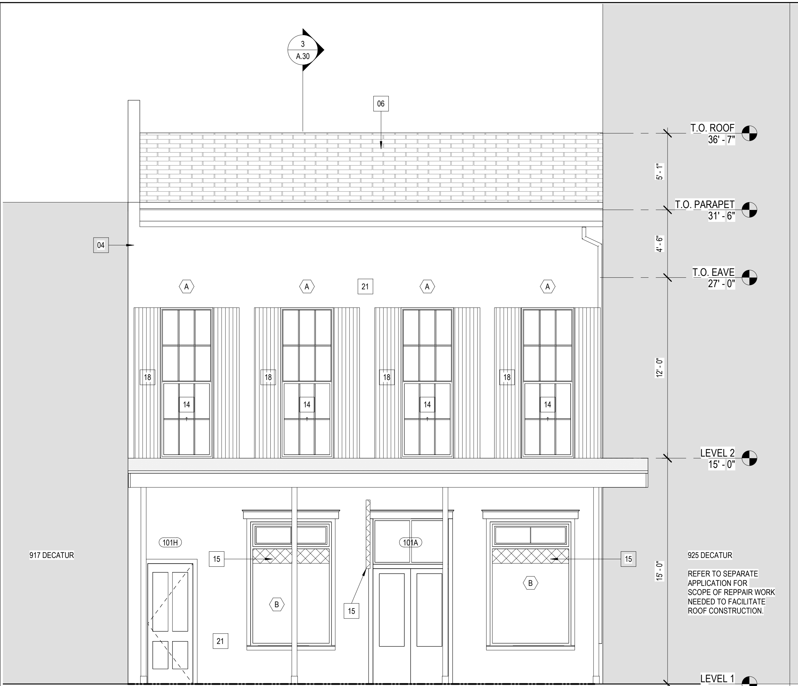
1 DECATUR STREET ELEVATION SCALE: 1/4" = 1'-0"
